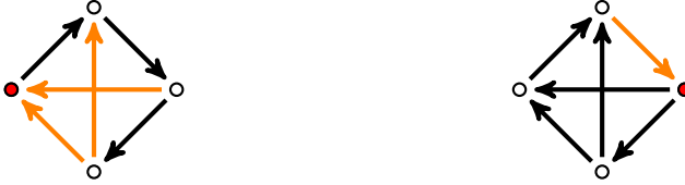
Figure 1: Two minimal feedback arc sets in a digraph D highlighted in orange. Drains are illustrated by red vertices.
