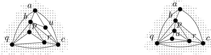
(a) Graph before the vertex relocation move with vertex  $u$  in face  $\{a, b, c\}$ .
