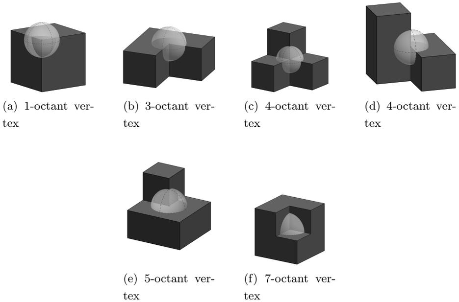
Figure 6: Vertex classification for orthogonal polyhedra.
