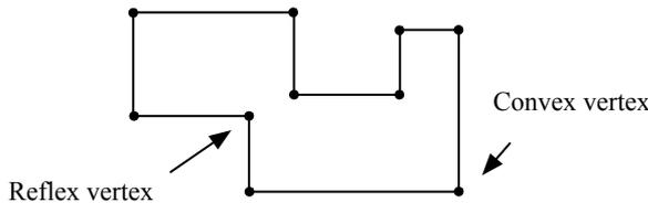
Figure 4: Reflex and convex vertices of an orthogonal polygon.
